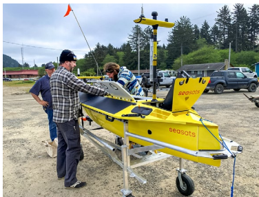
SeaSats “Lightfish” Autonomous Surface Vehicle with water sampler
